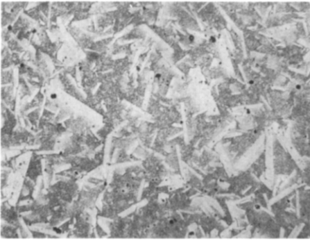
Fig. 9. Microstructure of beta-alumina with a duplex morphology of coarse grains ( \sim 100 \mu\text{m} ) in a fine-grained matrix, \times 80 .
